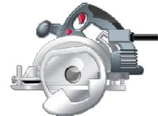
Angle grinders are not recommended as they often provide a poor cut and are less safe to operate than circular or drop saws.
